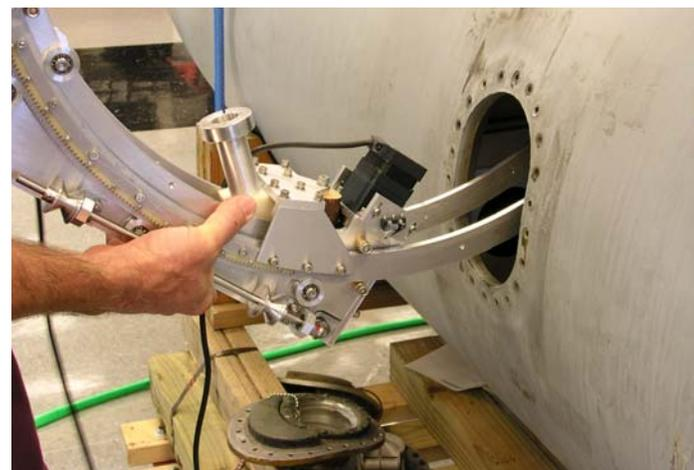
The TCAT, Texas A&M Engineering, and Georgia Tech Research team utilized their extensive experience and expertise in ultrasonic NDI techniques and mechanical engineering to produce a robotic device that could be inserted into a fuel tank, then manipulated to inspect the tank inner surface. The result was a solution to a problem of immediate concern to Warfighter readiness.
